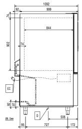
Drain FΙ Electrical inlet (power) Refrigerant Outlet
